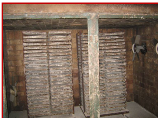
Figure 3.13: Operation of conventional tray dryer system at Chemical unit
