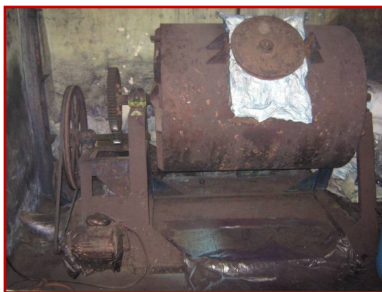
Figure 3.7: Conventional Position of motor in operation of ball mills in typical chemical unit
